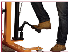
Hydraulic pump action
